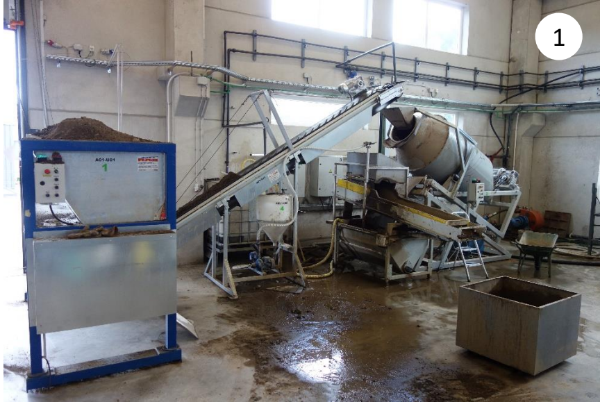
Soil rinsing, separation
