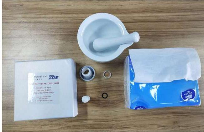
2. Take the Polypropylene film and lay it over the bottom opening on the sample cup.
