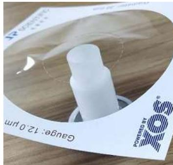
3. Place sample ring on the film and slide it over the sample cup. This will capture the film under the ring and around the sample cup opening. Slide the ring down half way, so it can be easily removed later. If there are any wrinkles or tears, this step should be repeated.
