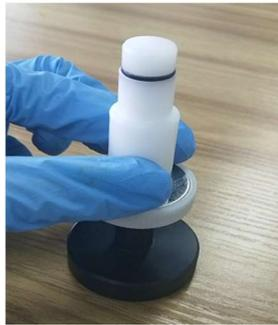
3. If the o-ring is dirty, replace it with a new o-ring after cleaning plunger.
