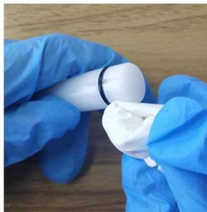
6. Rinse the inside of the sample cup and the sample pusher with isopropyl alcohol (IPA) and let air dry.
