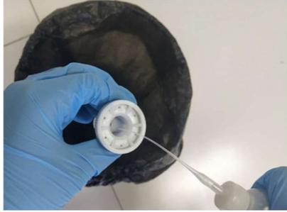
7. Once fully dry they are ready to be used again. If needed, install new o-ring on plunger
