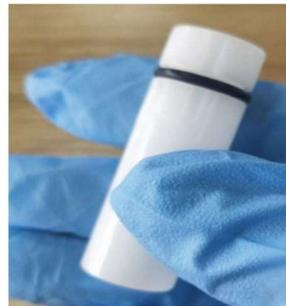
9. Place the plunger into the sample cup, o-ring side first.
